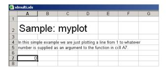
This procedure plots a line from 1 through 4 in a MATLAB Figure window. This graphic can be manipulated as if it were called from MATLAB directly. The calling cell contains 0 because the function does not return a value.
