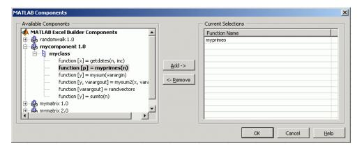
The Component Browser lists each component by name and version. Expanding a component reveals the class name at the next level. You can also expand the class to reveal the MATLAB functions that make up the class methods.
