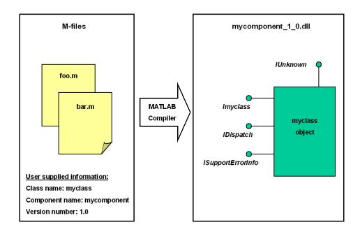
The process of creating an Excel Builder component is completely automatic from a user point of view. You specify a list of M-files to process and a few additional pieces of information, such as the component name, the class names, and the version number. The build process involves the following steps:
